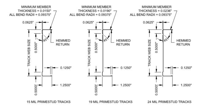
TRACK WEB DIMENSIONS (INSIDE DIMENSIONS):  $1^{5/}_{8"},\,2^{1/}_{2"},\,3^{5/}_{8"},\,4",\,\text{and }6"$
