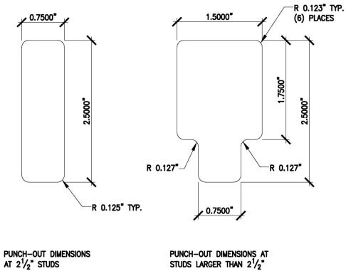
PUNCH-OUT DIMENSIONS AT STUDS LARGER THAN  $2^{1}/_{2}$ "
